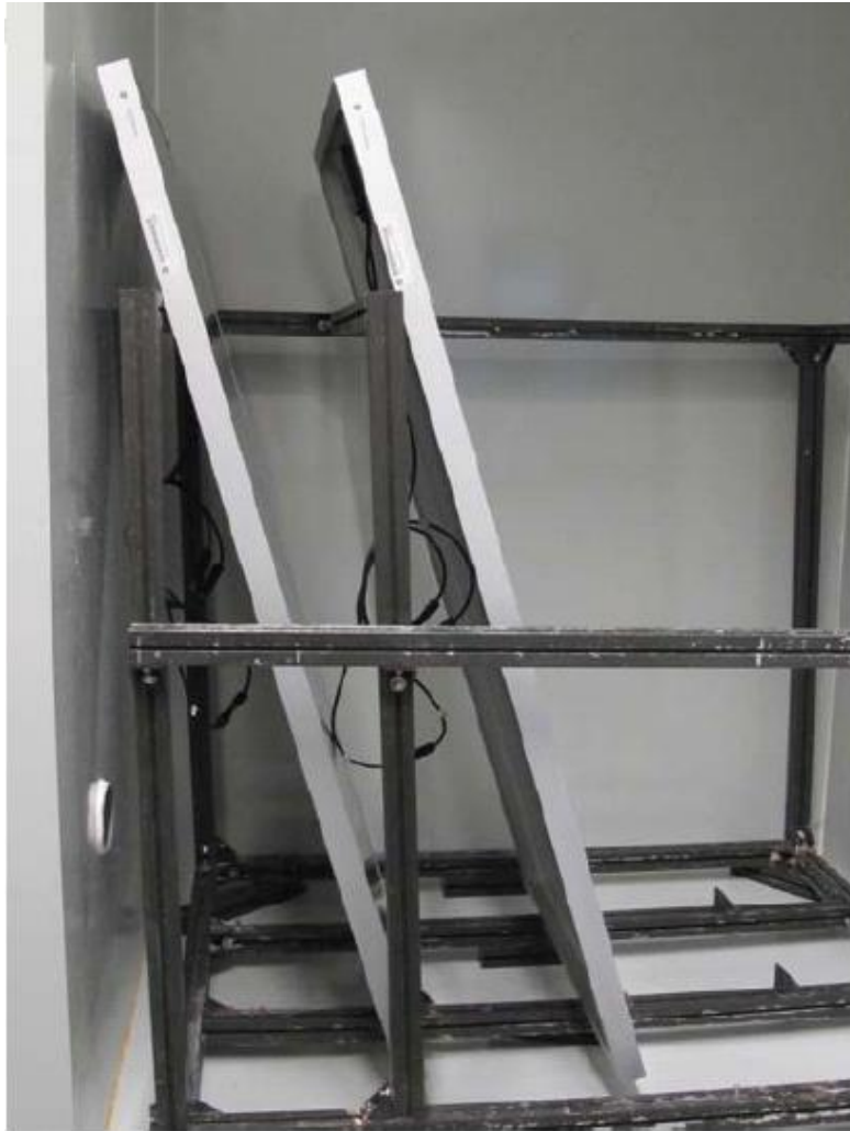
Sample 1 and sample 2 in salt mist test chamber
