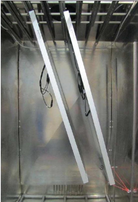
Sample 1 and sample 2 in ammonia test chamber
